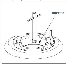
Figure 14 Triple ring wok burner
